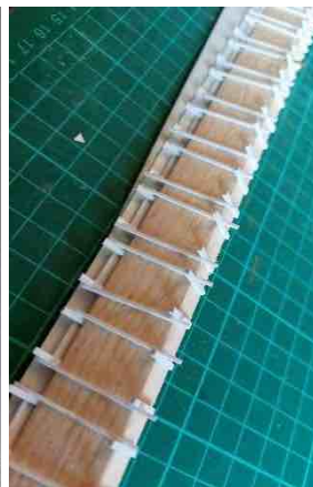
panelen in de lijmmal
